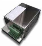
The W Marine 10 and GSR 12-24 are a solar charge controller with "MPPT step up and step down" technology. That technology can drive panels with a rated voltage above or below that of battery optimizing the charge. A technology that makes easy every installation in all types of marine applications.
